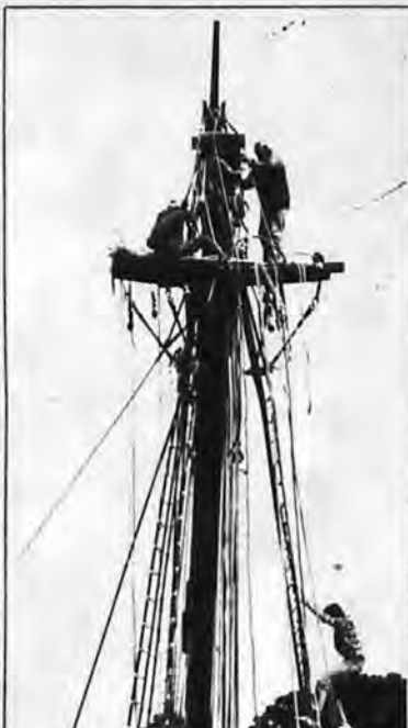
Ted McCutcheon (top right), Charlevoix boat builder, prepares the rigging on the 90-foot mast of the Welcome , a replica of a 1775 British sloop. The Welcome was in Charlevoix this spring prior to being sailed to Mackinaw City where it is kept on display. McCutcheon built the 45-ton replica beginning in 1973. It was first launched in 1980.
